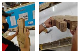
Visual Checking of the L-marking guide before bundling. (Up/Down & Left/Right)
